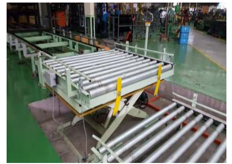
Transfer Process Systems
