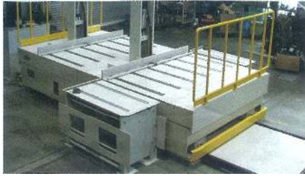
Quick Die / Mold Changing System for Injection Machine
