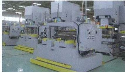
Quick Die / Mold Changing System for Sheet Metal Press
