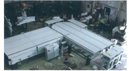
Quick Die / Mold Changing System for Hot Forging
