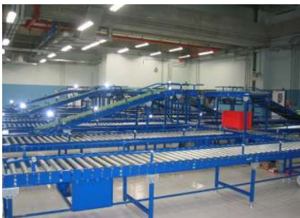
Multilevel Distribution Systems
